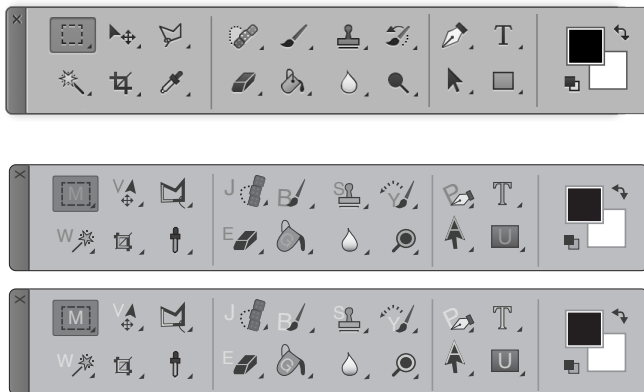
Figure 6. Possible adaption of the Adobe Photoshop CC 2015 interface using IconHK. Top: default toolbar. Middle & Bottom: the adapted toolbar integrating IconHK principles at two different levels of magnification. All buttons embed their associated hotkey, except the Blur button (water drop) which lacks a shortcut.
